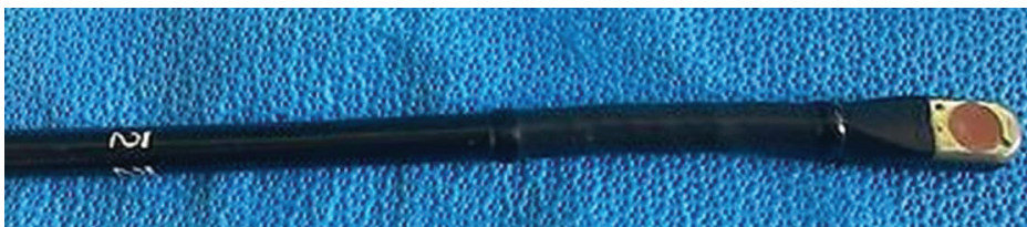
Transducer damage due to impact on the distal tip
