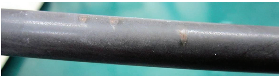
Biofilm formation due to improper cleaning technique
